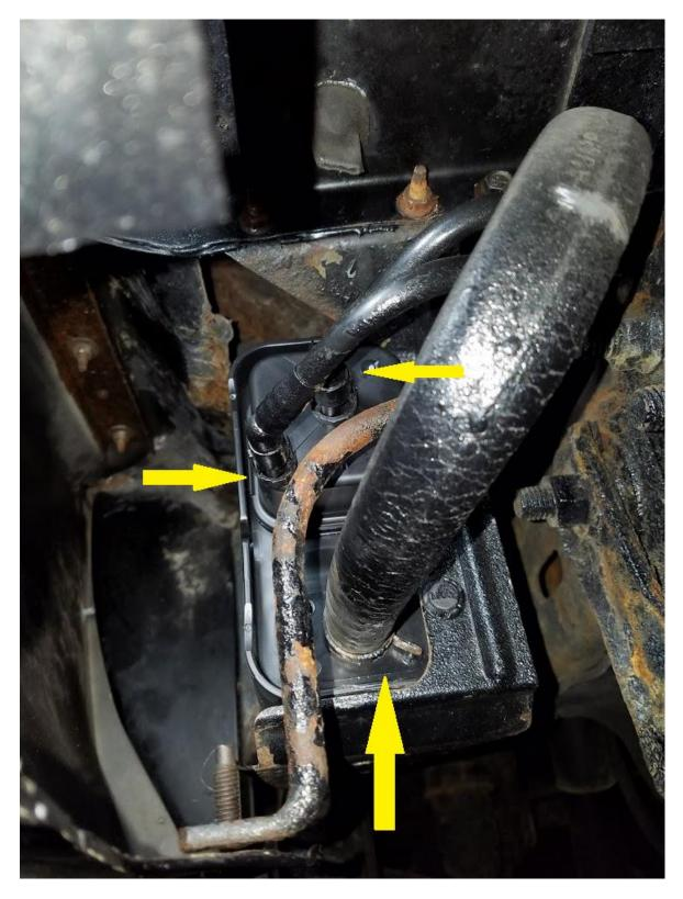
3) With the hoses removed you can now remove the four bolts that hold the frame that the canister sit in. Depending on the kind of mud flaps you have on, it is easier to remove it to get at the two from bolts from the canister frame. I only needed to remove two screws and move the flap down to remove these bolts.
