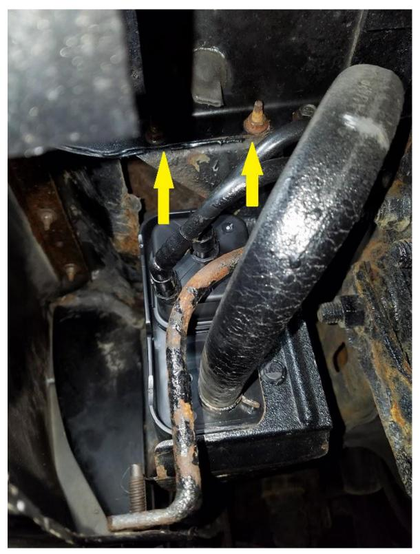
5) This is a bracket that holds the bumper panel to the frame to prevent wiggling and to add more support. The bolt was rusted and I sheared off the head when I tried to remove it. This bracket does not need to be removed however it makes access easier. I had a 10mm stainless screw and bolt handy so I replaced this.
