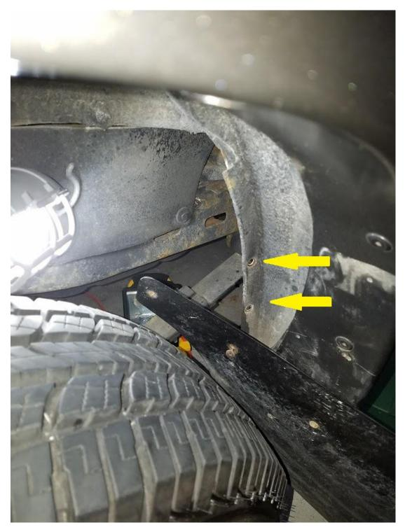
4) You can now move to the canister and remove the remaining two bolts. After these are removed, the frame with canister will come out.
