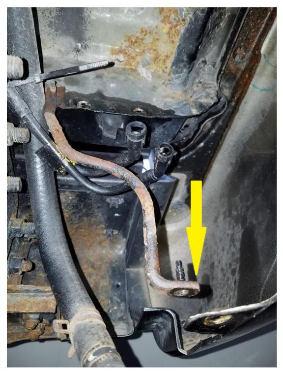
6) Do yourself a favor now that the canister is removed and clean up the area. I took a wire brush and cleaned up some of the dirt and rust that was under there. I sprayed some black paint primer and after it dried I sprayed some black rubber undercoating. I know it may not make the biggest difference but I feel better! Sorry, I did not take any after pictures of this  $\otimes$
