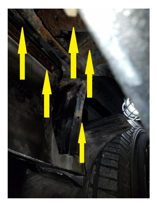
7) With the canister and frame removed, there are a few tabs that are bent in to hold the canister to the frame. You will need to pry these tabs out with a flathead screwdriver. Note which way the canister goes into the frame before removing.
