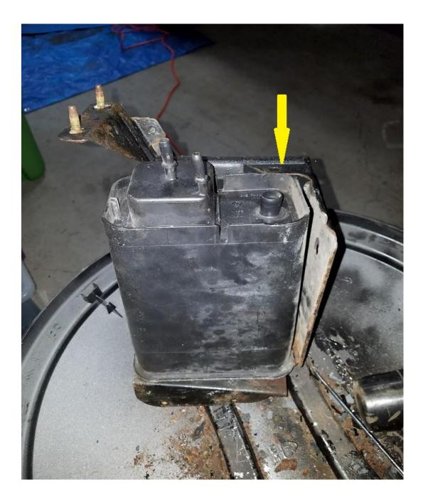
8) At this point, do yourself a favor again and clean up the canister frame. I took a wire brush and got the rust off and sprayed it with some black primer and after it dried, some black rubber undercoating. The reinstall is virtually the same as removal. It is easier at this point to bolt back the bumper panel before reinstalling the frame with the canister in and reattaching the hoses back to the canister.
