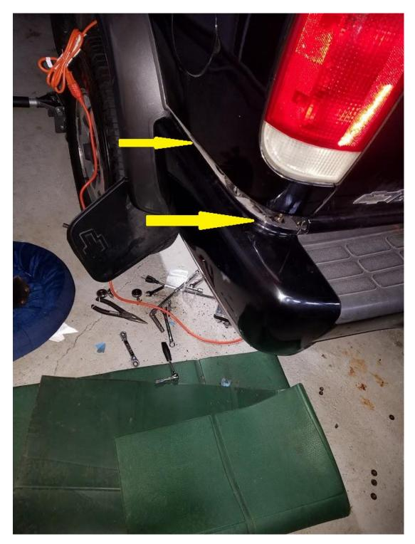
2) Once you remove the fender bolts you will have better access to the canister. It is easier to disconnect the three hoses that go into the canister before trying to remove it. They are simple to remove as you will need a pair of pliers for the larger hose. For the smaller hoses, note what port the connect to before disconnecting as you will only need to pinch these off by hand. Be careful not to break the pinch connectors as these are what hold the hoses to the canister.
