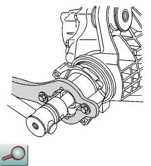
14. Install the <u>J 8614-01</u> onto the pinion yoke as shown.
