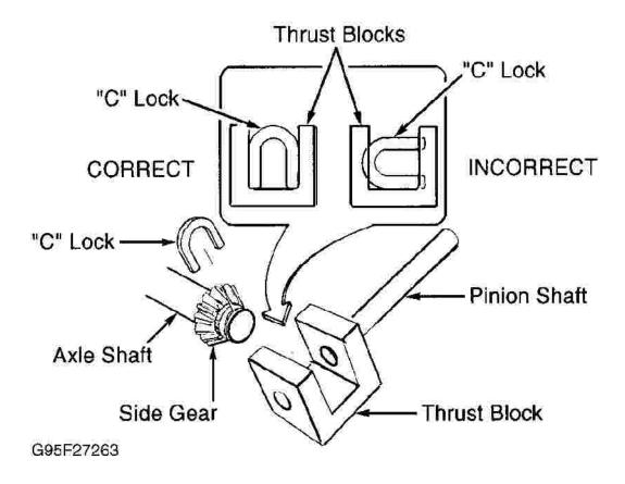
Fig. 2: Removing "C" Lock From Locking Differential Courtesy of GENERAL MOTORS CORP.
