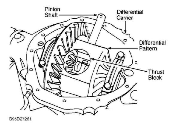
Fig. 1: Removing Axle From Locking Differential Assembly Courtesy of GENERAL MOTORS CORP.
