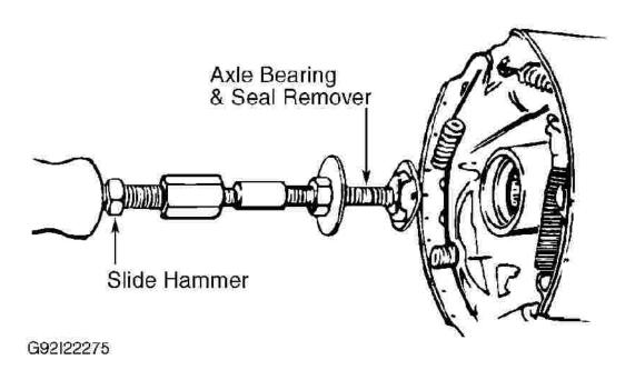
Fig. 3: Removing Axle Bearing & Seal Courtesy of GENERAL MOTORS CORP.
