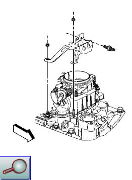
10. Remove the accelerator cable bracket from the throttle body and the intake manifold.
