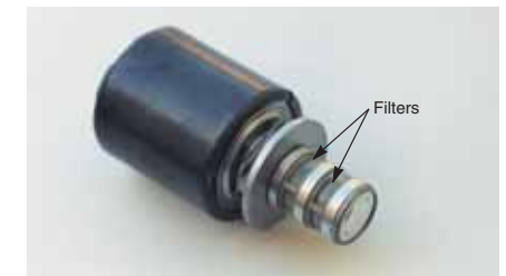
Figure 14-4. The valves of a solenoid are machined to extremely small clearances and cannot tolerate the presence of even the smallest particle of dirt or metal. Most transmission solenoids are equipped with small filters to reduce the possibility of contamination. These filters can plug up, especially if other transmission or transaxle parts have failed.
