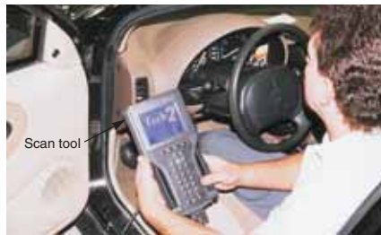
Figure 14-9. Scan tools can be used to retrieve trouble codes and obtain other information about the operation of an electronic transmission or transaxle.
