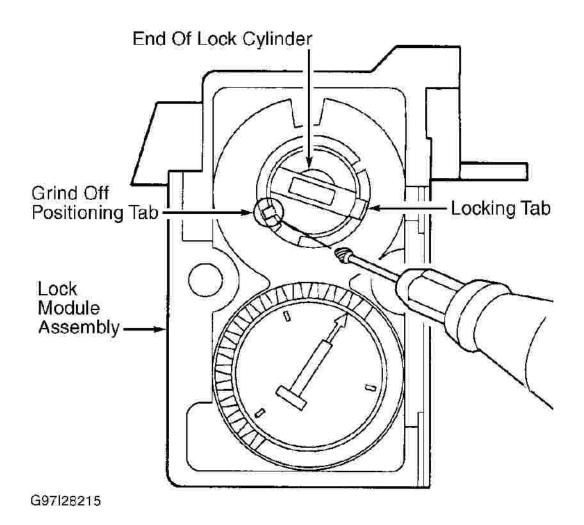
**Fig. 4: Removing Lock Cylinder Positioning Tab Courtesy of GENERAL MOTORS CORP.**
