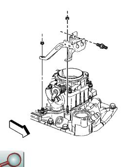
20. Remove the accelerator cable bracket from the throttle body and the intake manifold.
