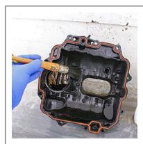
I cleaned up the upper intake manifold with mineral spirits and a brush. I also used carburator cleaner to clean the deposits from around the throttle plate.
