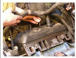
I set the valve cover in place and installed the bolts with a 13mm socket.
