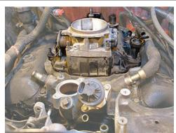
At this point the upper intake manifold and throttle body were ready to be removed.
