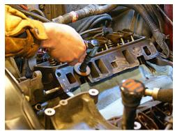
Before replacing the valve covers or the intake manifold, I cleaned up the mating surfaces with a die grinder and a 3M Roloc abrasive disc.
