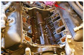
This is the engine with the lower intake manifold removed.
