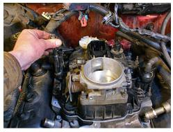
Installing the upper intake manifold was not as straightforward as you would think. The manifold "hung up" on the central fuel injection unit. (It did the same during removal.) When I set the manifold in place, it was resting on the injection unit but there was a 1/4" gap between the upper and lower manifolds.
