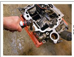
I set the intake manifold on a milk crate and used a die grinder with a Roloc disc to clean up the mating surfaces. First I did the top side.
