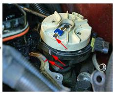
To make the match-mark on the lower intake manifold, I used a **red marker AND a scratch-awl**. It's important to make a decent scribe mark in the metal, because after the manifold is cleaned up with an abrasive disc the mark will be hard to see.
