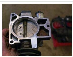
After removing the throttle body, I cleaned the bottom surface with a Roloc disc on a die grinder.
