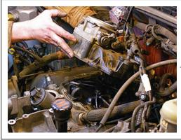
Then the upper intake manifold was completely free.
