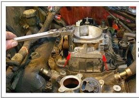
There were two long bolts at the front of the throttle body, and two regular bolts at the rear of the upper intake manifold.
