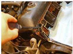
I spent a few minutes with a shop vac and a small screwdriver to scrape off any dirt and suck it into the vacuum cleaner. I want to avoid getting too much grit in the crankcase.
