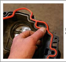
$\ensuremath{\mathrm{I}}$  installed the new gasket on the bottom of the upper intake manifold.
