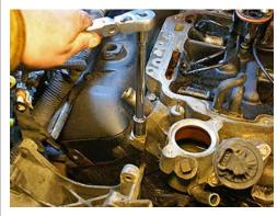
I removed the bolts with a 13mm socket, long extension and ratchet. First I **loosened each bolt** and then I removed them all.
