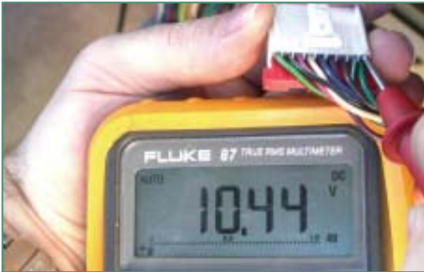
Figure 9: Check DRAC harness connector terminal C15 (Speedometer Signal) for 10 -12 volt pull up
