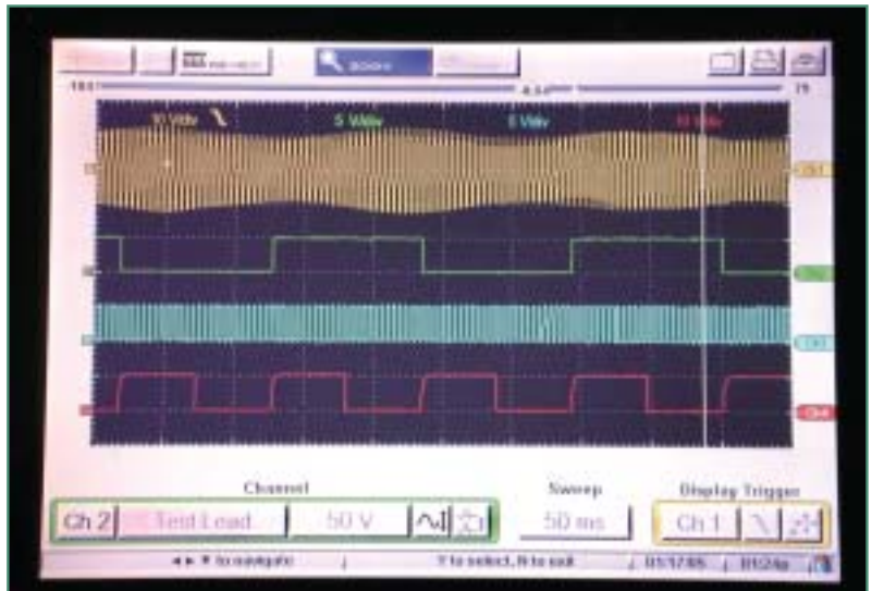
Figure 12: After zooming out, we can view more cycles of the Vehicle Speed and Speedometer signal waveforms
