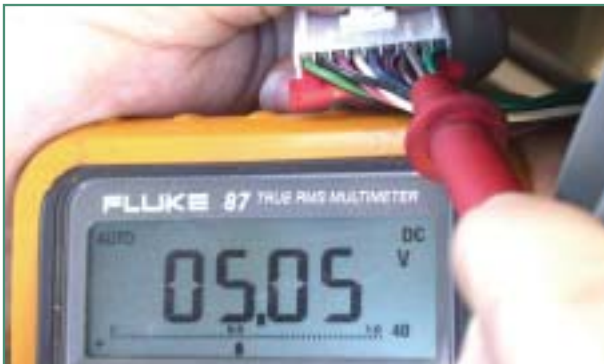
Figure 7: Check DRAC harness connector terminal C13 (Output Speed Signal) for 5 Volt Pull-Up
