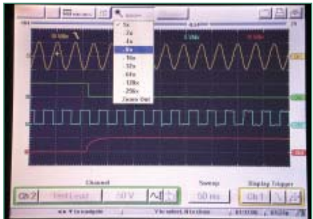
Figure 11: Selecting the 'Zoom Out' 8x function to view slower signal components.
