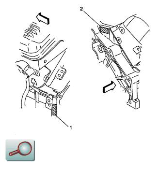
The Vehicle Identification Number (VIN) Derivative is located on the left side rear of the engine block (1) or on the right side rear (2) and typically is a nine digit number stamped or laser etched onto the engine at the vehicle assembly plant.
