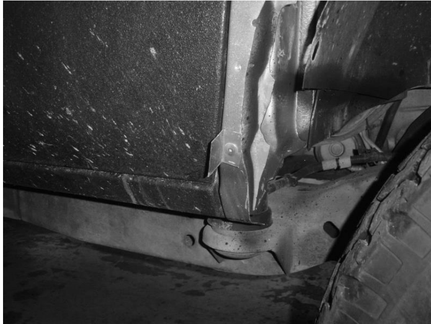
Another angle showing the tab at the bottom of the front fender (Passenger Side)
