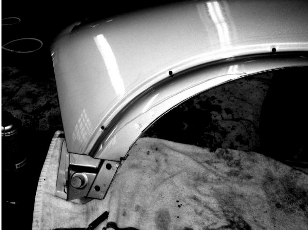
These pictures show the front flare front cut lines. The large stud at the bottom left of the picture will be retained, but the two holes right of the stud will be removed.
