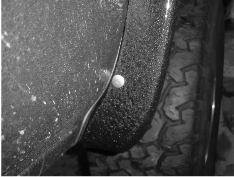
Close up of the rivet at the back of the front flare. Note that we did not use trim on these flares because they were coated in Line-X Bed coating
