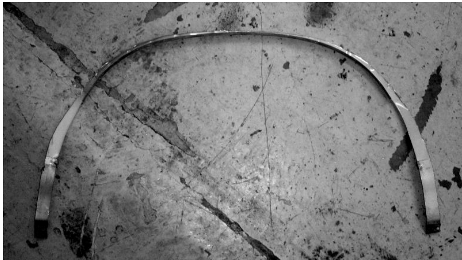
This is the piece of metal you will be removing on a ZR2 pickup bed. It should be 1.50” on each side and only 1.00” at the top.
