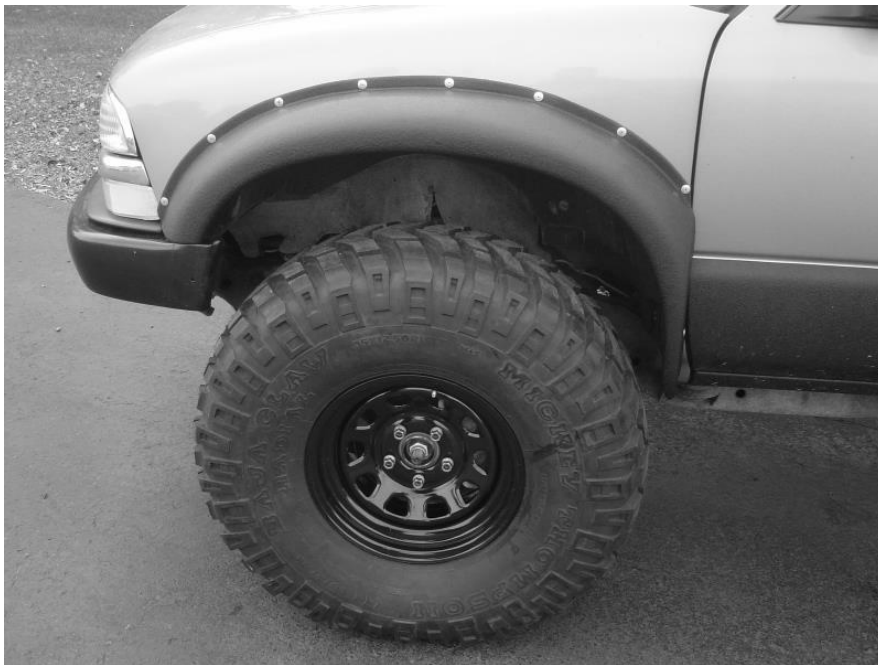
The Front Flare Installed. Try to keep the rivet spacing as even as possible for a clean look.
