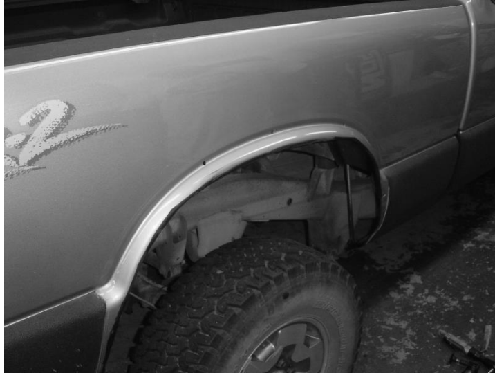
This picture shows a ZR2 Pickup Rear bedside with the flare removed
