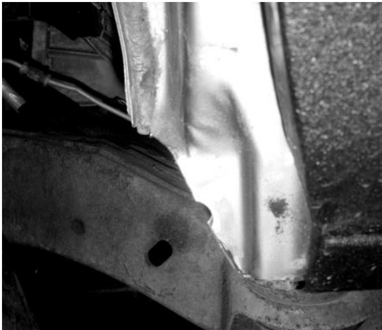
A picture showing the tab after removal (Driver's side)
