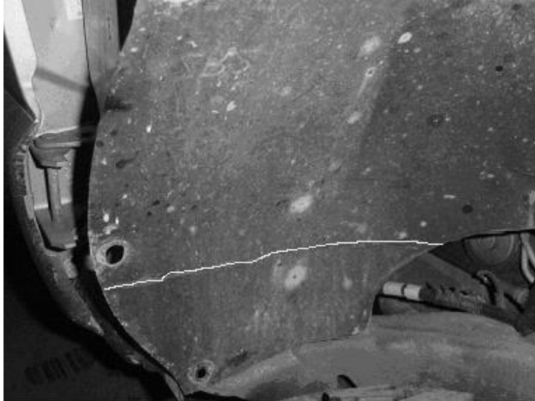
This picture shows the cut line for the inner fender liner. (Passenger side)
