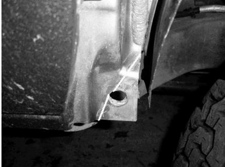
This is the cut line for the fender mounting tab on the cab itself. (Passenger side)
