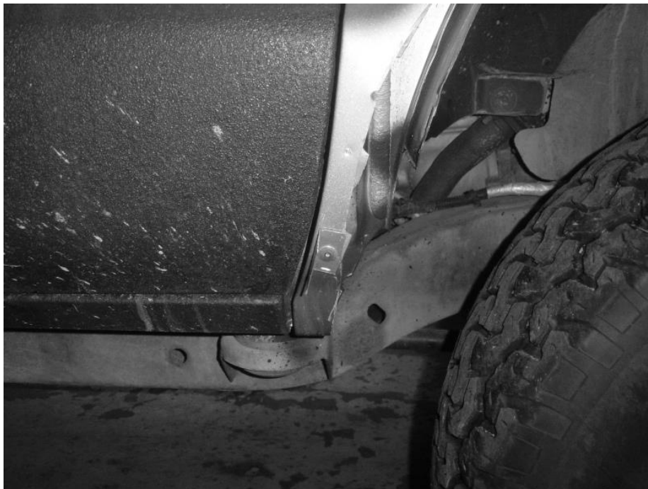
The bracket should be about 3/16" from the door gap. The flare itself should be flush with the door gap after installation.
