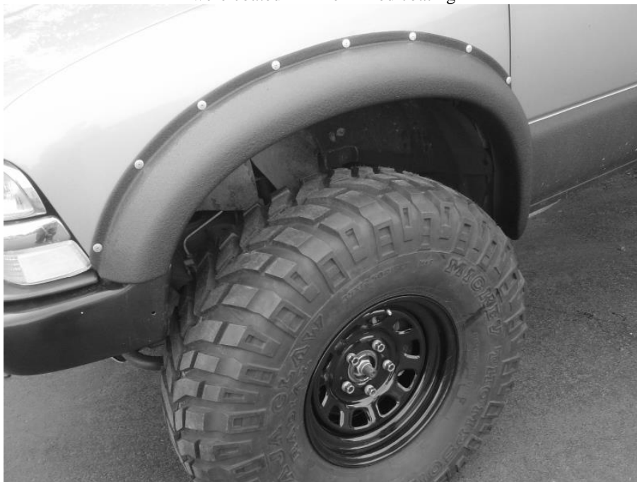
Close up of the rivet at the back of the front flare. Note that we did not use trim on these flares because they were coated in Line-X Bed coating
