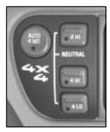
The transfer case switches are to the right of the steering wheel on the instrument panel. Use these switches to shift into and out of four-wheel drive. You can choose among four driving settings:
