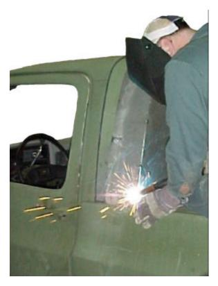
Photo 5 – The cap back panel is tack welded to the cap top extension. Once securely tacked together, remove the components to finish the welding process off the vehicle.
