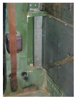
Photo 3 – Sheet metal screws hold the mounting angles to the vehicle's side panels.
