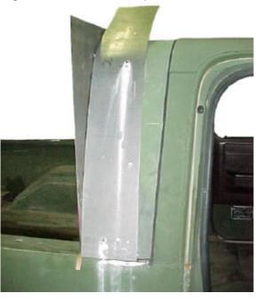
Photo 4 – The steel panel extension to the cab top is wrapped and bolted to the modified cap. The cap back can be used to locate it fore and aft.
