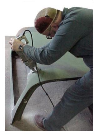
Photo 1 – The front of the cap is sawed off.
